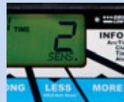
**EXCLUSIVE! InfoTrack™** technology on Titanium helmets allows the lens to track arc time while under the hood. Includes a digital clock display with the ability to set an alarm or timer.
