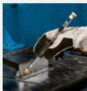
**Rugged ArcStation™ base** features a 1/2-inch reversible steel table top and ships complete with drawers, gun holder, quick-release clamps and heavy-duty casters for mobility.
