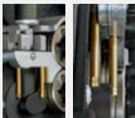
**Ultra-low drag inlet guide pins** make loading the wire easy and does not deform the wire on the way into the drive rolls improving wire feeding performance.
