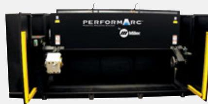
**Dual head and tailstock/single-, dual- or triple-robot configuration**
