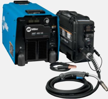
**ArcReach™** Remote control of the power source without a cord. With an ArcReach-equipped SuitCase® feeder and power source you can change the output voltage at the feeder, and save a trip to the power supply. No extra control cable to purchase, maintain, string or unstring – saving time and money.
