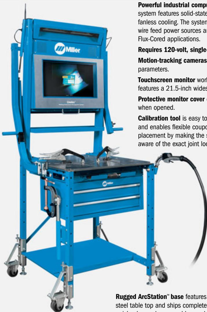
**Powerful industrial computer** at the heart of the system features solid-state technology and filterless, fanless cooling. The system is compatible with Miller® wire feed power sources and is capable of MIG and Flux-Cored applications.
